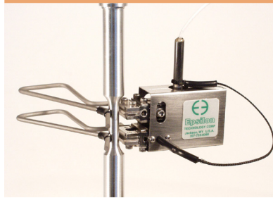
Model 4030 with 0.5 inch gauge length
