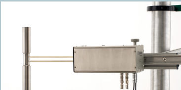
Model 7650A extensometer with rigid load frame mounting
