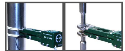
Rubber band and spring attachment options included with Models 3442 and 3542
