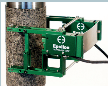
Model 3542RA1 extensometer with 50 mm gauge length
