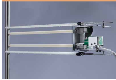
The Model 3448 is self-supporting using reusable ceramic cords
