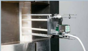
Self-supporting Model 3448 with clamshell-type materials testing furnace
