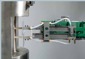
Model 3648 with 1 inch gauge length
