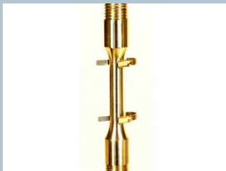
Laser extensometer high temperature clip-on reflectors
