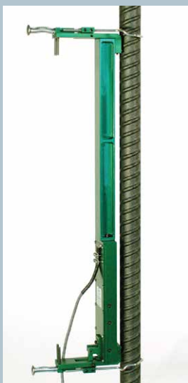
Model 3543 with 12 inch gauge length
