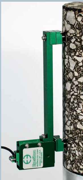
Model 3909-0400 with 4 inch gauge length
