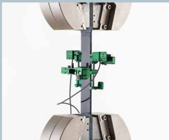
Model 3442AVG extensometer 3442-050M-025M-ST
