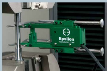
Model 3542 with 25 mm gauge length
