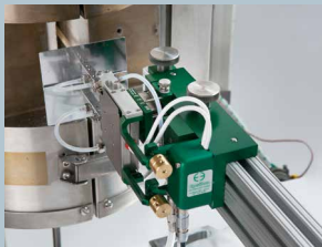
Model 3549 with 25 mm gauge length
