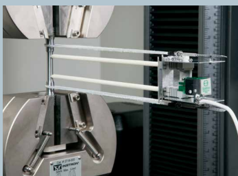
Model 3448 with 25 mm gauge length and 20% measuring range
