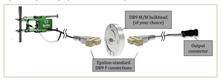
The solution above provides for maximum flexibility and interchangeability (with disconnects on both sides), and reduces immediate and future service costs (using Epsilon-standard connections, with shunt calibration references).
