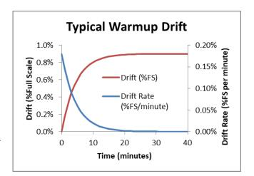
**Example 2:** A creep test lasting 10 minutes is performed after allowing the system to warm up for 10 minutes. The test elongation is 1.0% of sensor full scale, and drift during the test is 0.1% of sensor full scale. The measurement error is: 0.1%FS / 1%FS = **10% of reading**.
