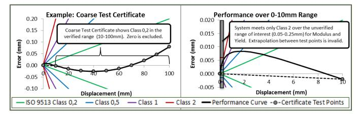
In this case, the measurement of interest is yield strength, which will be measured from 0.05-0.25mm range. A closer look at the true performance curve reveals that the extensometer meets *only class 2 over the range of interest*. The extensometer does not meet the required class for this measurement, despite a "Class 0,2" test certificate. <u>The test certificate from 10-100mm cannot be extrapolated to the 0-10mm range</u>.
