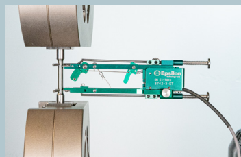
Model 3742 with 25 mm gauge length and +25 mm / -5 mm measuring range
